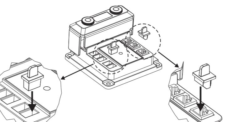
Please see the above illustration on how to cover unused ports of the active shunt module. A selection of rubber cover parts is included in the package.
