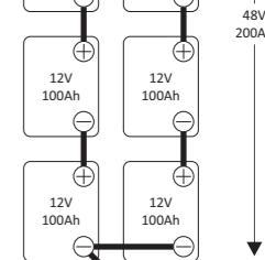
**Always connect the battery negative cable last when the installation has been completed.**
