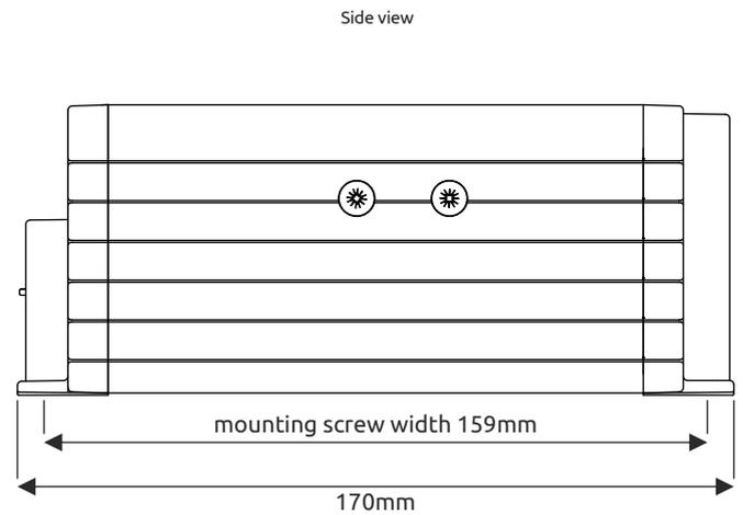
Measurement units: millimeters
