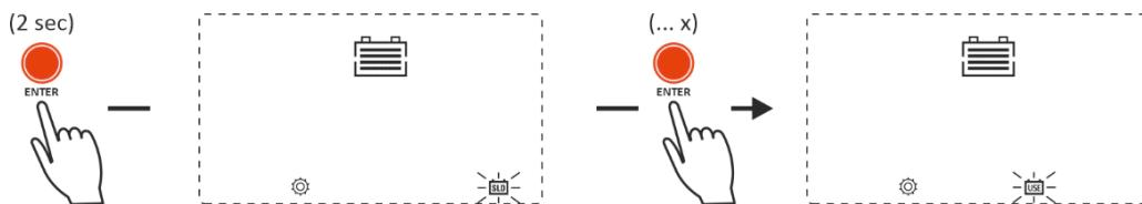
After the ENTER key has been pressed a number of times to select the USE battery type, press the SELECT key to jump to the system voltage selection and make sure the correct system voltage is selected as in the example below:
