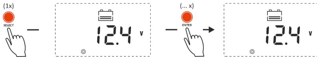
This parameter represents the voltage value at which the activated alarm relay will de-activate again, besides clearing the undervoltage alarm message. It can be edited by short pressing the ENTER key each time to increase the value by 0.1V. This value must always be higher than the Undervoltage alarm relay trigger voltage.
