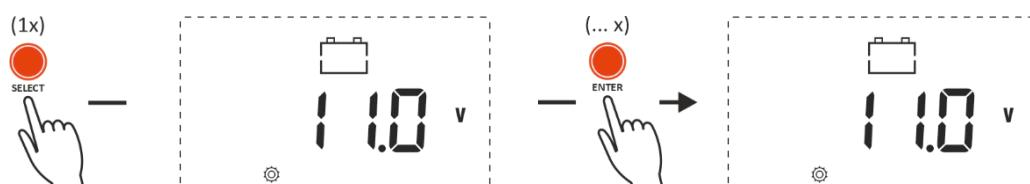
This parameter represents the voltage value at which the undervoltage alarm relay will be activated. It can be edited by short pressing the ENTER key each time to increase the value by 0.1V. This value must always be lower than the Undervoltage alarm off value.
