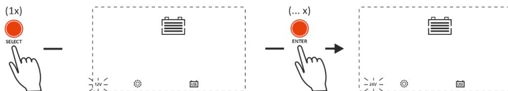
In this example a 24V system voltage is selected. When the SELECT key is pressed the first voltage parameter (Equalize charge voltage) is shown, see below:
