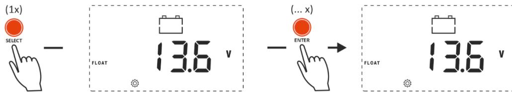
This voltage can be edited by short pressing the ENTER key each time to increase the value by 0.1V. When 17.0V is reached, the voltage value will jump back to 9.0V and can be increased again.
